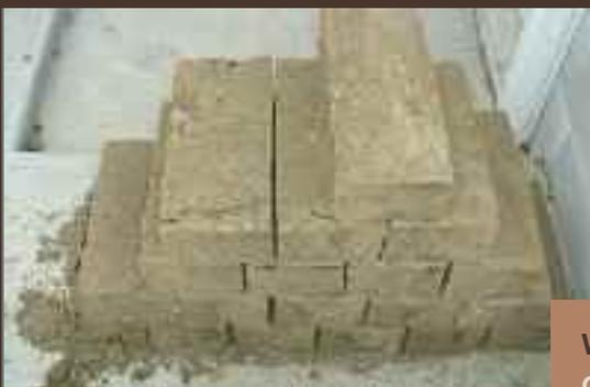
**Figure 5:** Crushing of bottom blocks after exposure to snow and rain (after 3 months)
